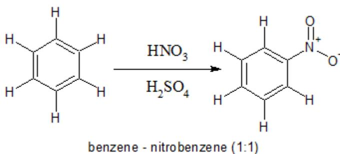
This is another way to show a chemical reaction. Chemists use this shorthand in organic reactions to minimize drawing carbons out and show the individual bonds. Each line represents a bond between atoms, where two bonds represents a double bond. Each intersection point represents one of the six carbons of benzene. Normally,
