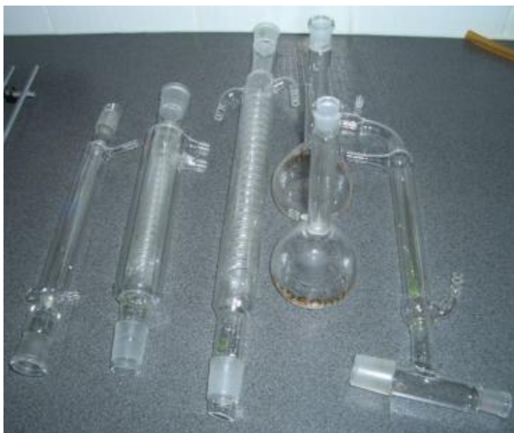
From left to right: Liebig condenser, two different styles of Graham coil condensers, two volumetric flasks, and a distillation head/condenser/vacuum take-off combination piece
