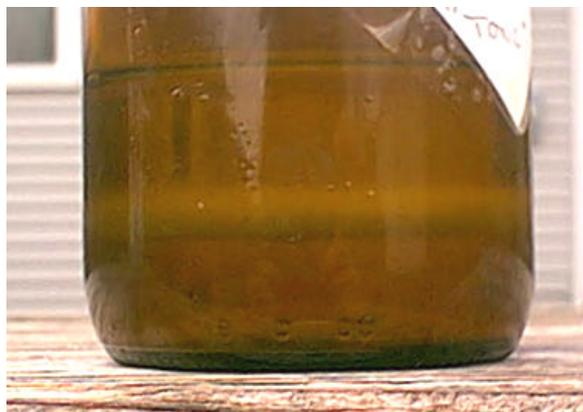
**Improperly stored chloroform, notice the layer between the water and the bottom chloroform layer.**
