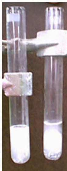
As shown in the above picture bases can rapidly attack some metals just as acids can. To the left in the above picture some aluminum turnings have been placed into a weak potassium hydroxide solution, to the right a weak acid solution is also attacking a similar amount of aluminum. Hydroxides can attack a number of metals, especially when hot and concentrated, however the reactivity shown with aluminum, zinc, and magnesium can be considered special cases for the common metals.
